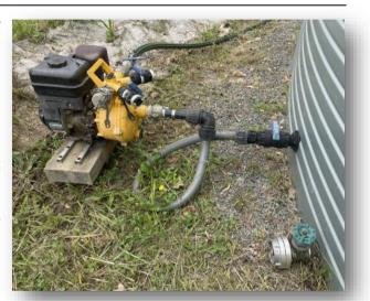
around' the property from both sides if needed using  $2 \times 60m$  configurations. We also have a portable Orange f/fighter pump and this can be hooked up to our other tanks as well as 1.5" riser with Storz fitting at the bottom of the orchard. We use this if doing pile burns or burning off the bottom paddock.
